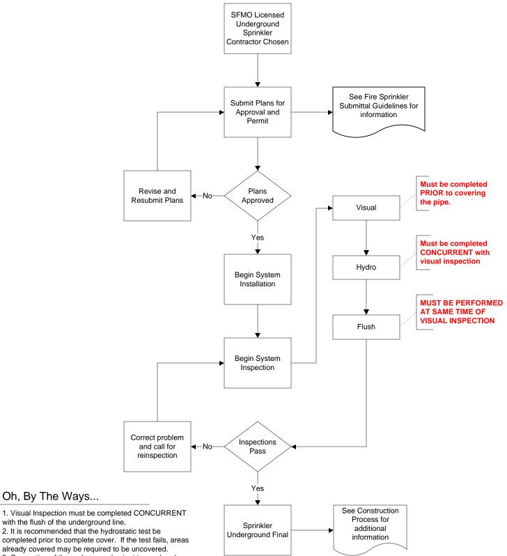
already covered may be required to be uncovered. 3. Connection of the underground spigot to overhead riser prior to flushing, or "stacking the riser", may result in the overhead pipe being required to be flushed.
