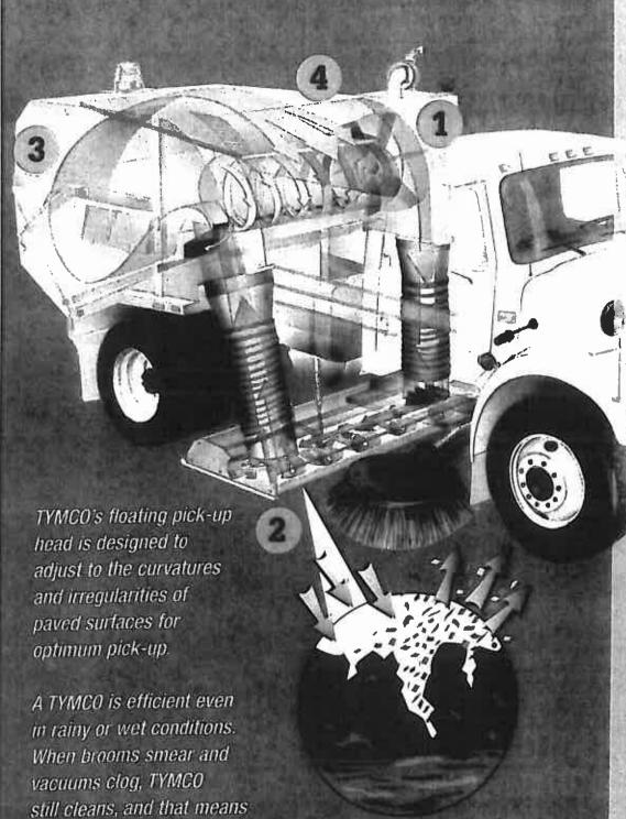
1. The closed-loop Regenerative Air System uses the force of a high velocity controlled jet of air created by the powerful blower wheel.
