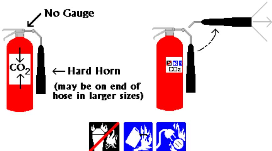
Carbon Dioxide extinguishers are filled with non-flammable carbon dioxide gas under extreme pressure. You can recognize a CO<sub>2</sub> extinguisher by its hard horn and lack of pressure gauge. The pressure in the cylinder is so great that when you use one of these extinguishers, bits of dry ice may shoot out the horn.
